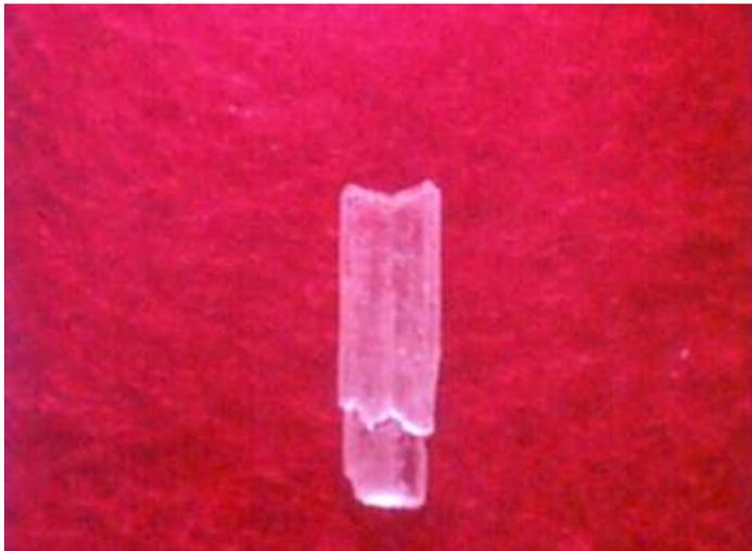
Fingernails have a Mohs hardness of 2.5, while calcium sulfate is 2 and calcium carbonate is 3. Here is a calcium sulfate crystal that has been scratched on the side with a fingernail to show that the crystal is softer than the nail:
