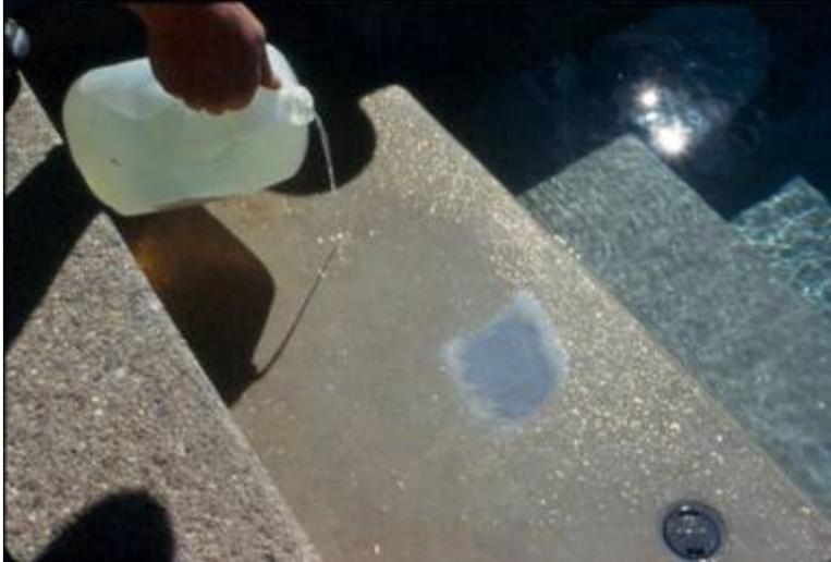
But when the acid hit the bare plaster, which contains calcium carbonate, it reacted, in the form of white effervescence:
